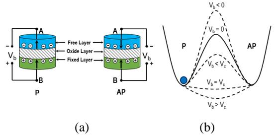
Figure 1: (a) VCMA-MTJ Structure, and (b) Energy barrier modification using VCMA Effect [1].
