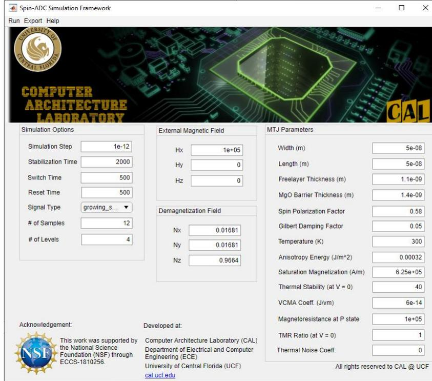
Figure 4: Spin-based ADC Interactive Simulation GUI.
