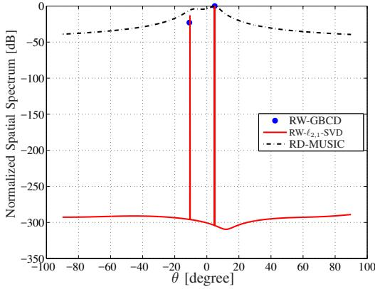
Fig. 5: Normalized spatial spectrum of RD-MUSIC, RW-GBCD and RW- $\ell_{2,1}$ -SVD for last iteration.
