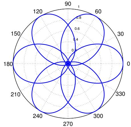
Fig. 1: Beampatterns of a 7-element ESPAR
