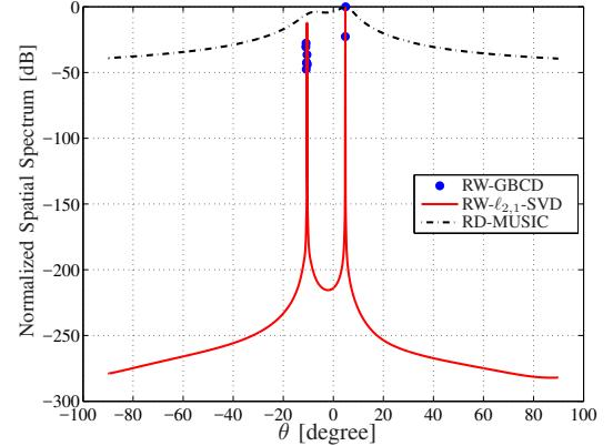
Fig. 3: Normalized spatial spectrum of RD-MUSIC, RW-GBCD and RW- $\ell_{2,1}$ -SVD for first iteration.
